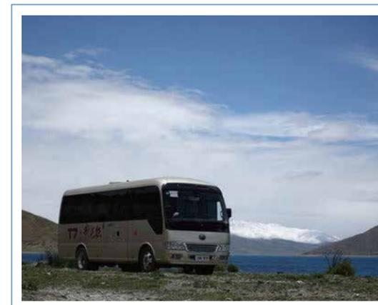
According to the bus maker, Yutong T7 adopts 6.0 liter V8 engine made by the US-based GM. With a horsepower of 315 (232 kilowatts) and a torque of 490 N·m, T7 easily climbs an uphill of over 20 kilometers. Moreover, the rotational speed of its engine stays between 1,500 and 2,000 RPM, showing high fuel efficiency level.
